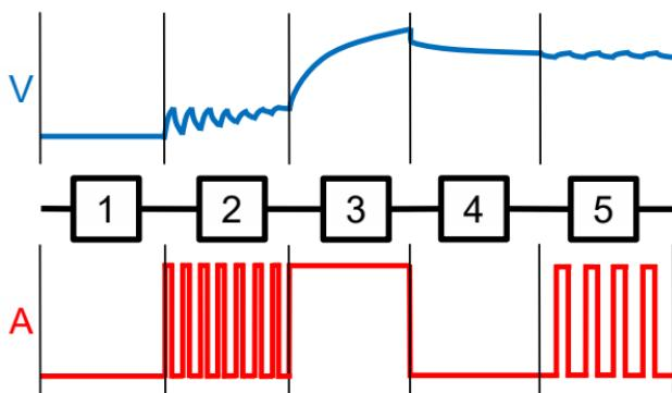
Step 1 / Battery check: after selecting the charging mode, the charger checks the status of the battery.
